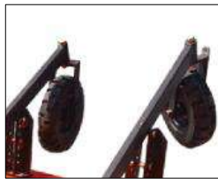
Tyre assembly for depth control
